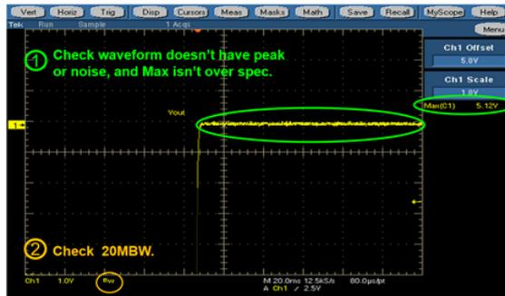
1. Check waveform does not have any peak or noise.
