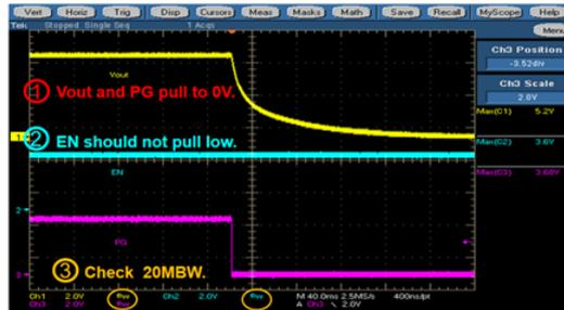
1. Check Vout and PG need to pull low to 0V. (check each IC spec)
